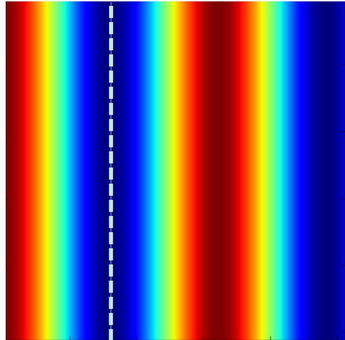
Can't tell the difference between a constant field ( $k_x=k_y=k_z=0$ ) and one varying transverse to the line-of-sight ( $k_x>0$  or  $k_y>0$ )
