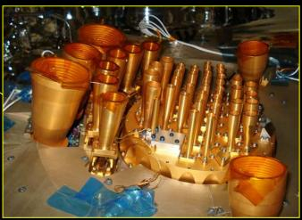
LFI Radiometers 30-70 GHz, T = 20 K
