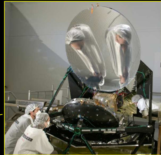
Planck Telescope 1.5x1.9m off-axis Gregorian T = 50 K
